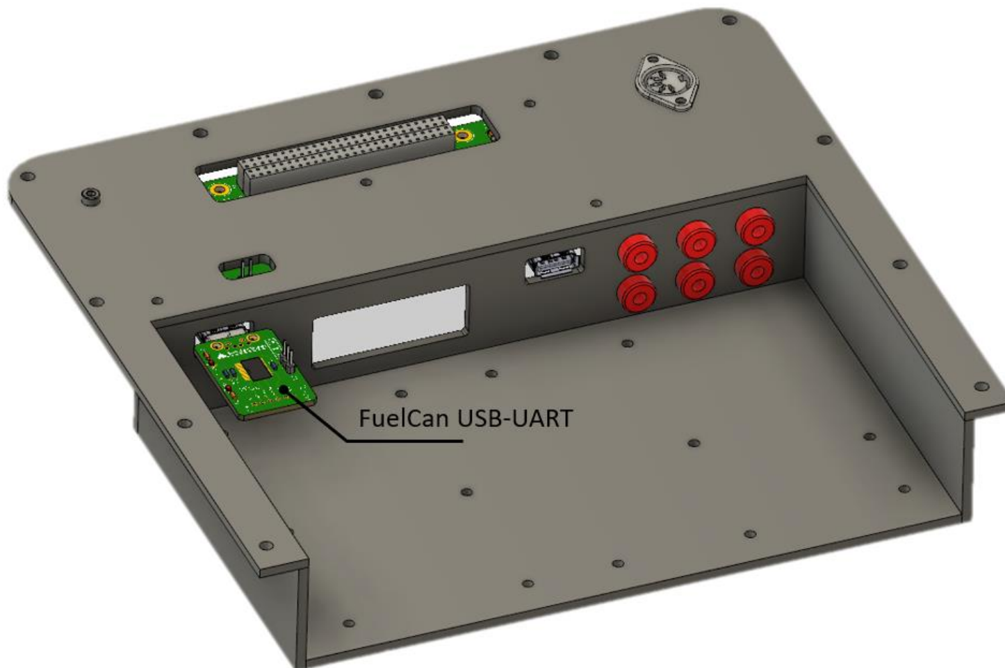
Figure 3. Installation of USB-UART in FuelCan™.
