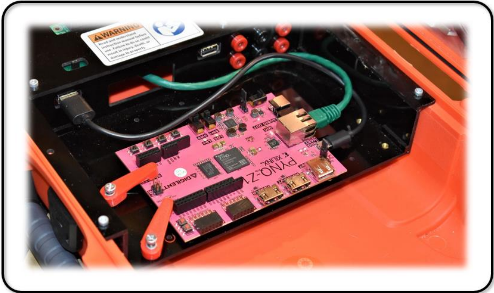
Figure 9. Mounting PYNQ™-Z1 with Hold-Down Clamps.
